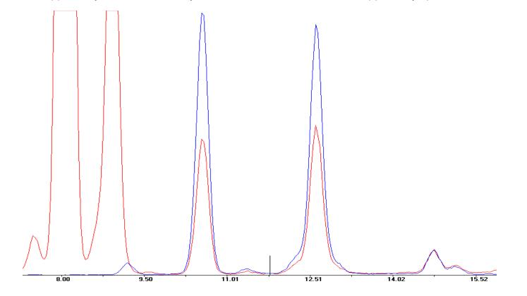
So in the case when just lead and copper are present you can use this information to determine whether the lead is on the surface, in which case the spectrum should look more like the blue spectrum above. This might indicate that the copper has corroded away leaving lead on the surface.
